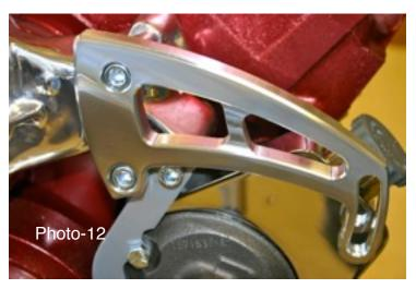
Check the distance between the front bracket and the power steering pump there should be a gap big enough to fill with one 3/8 washer. If the distance is greater it my be necessary to remove one washer from the rear of the lower rear support to move the pump forward this will achieve a movement of 3/32 on one inch.
