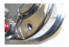
**Photo-8** Mounting the P/S. If your P/S pump came with a mounting stud at the rear lower 6 o'clock position in the the pump use a 11/16 wrench and remove it.
