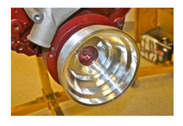
**Photo-2** Install the Water Pump Pulley (6322-A) and the pulley cover (314-A) using four 5/16 x 5/8 SHCS (S183).
